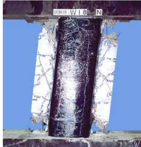
(b) Specimen strengthened by SR-CF system
